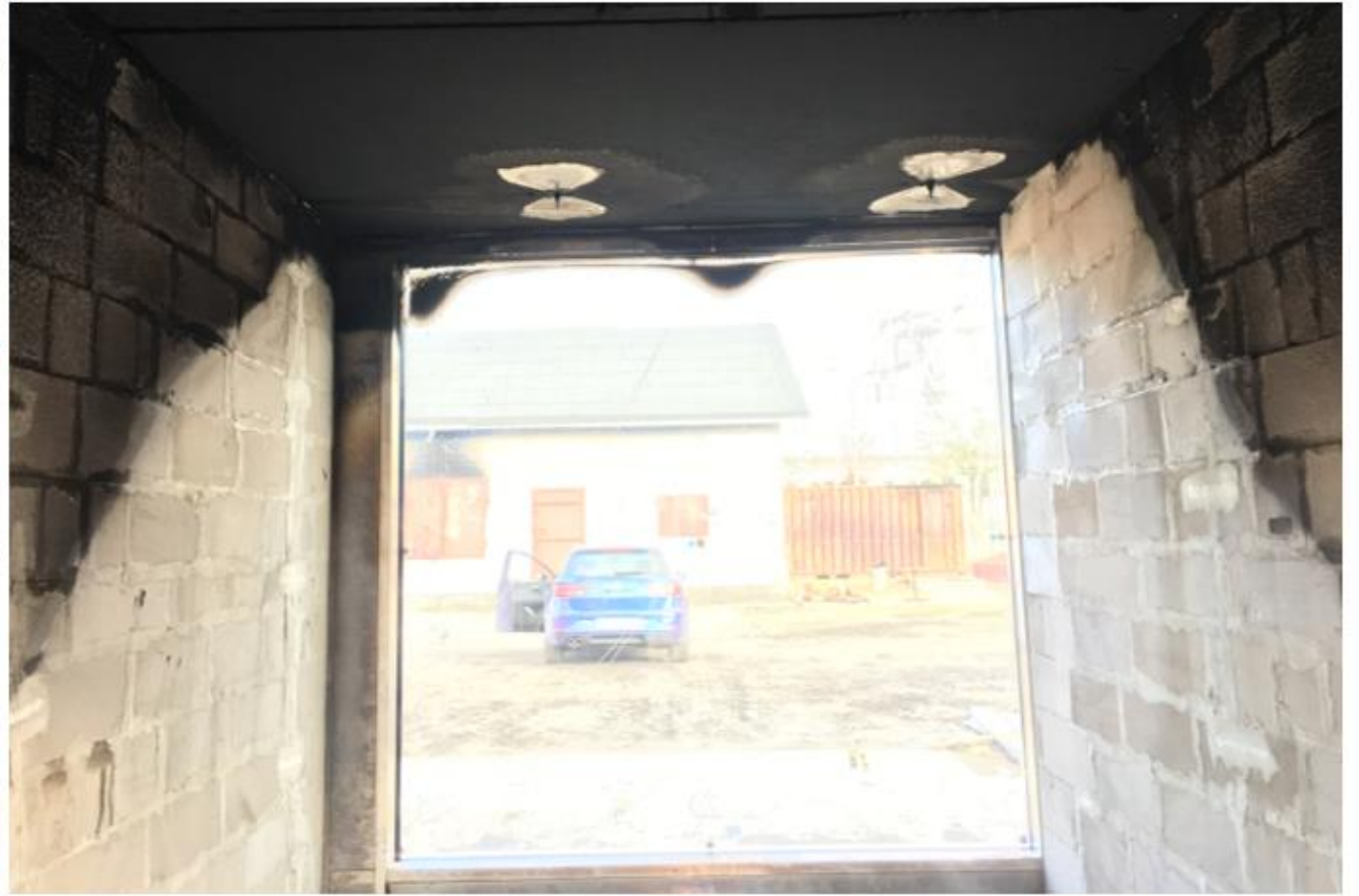
Figure 13. Soot deposition on the walls and the glazing of experiment #4, illustrating the range of water spray coverage in the compartment
