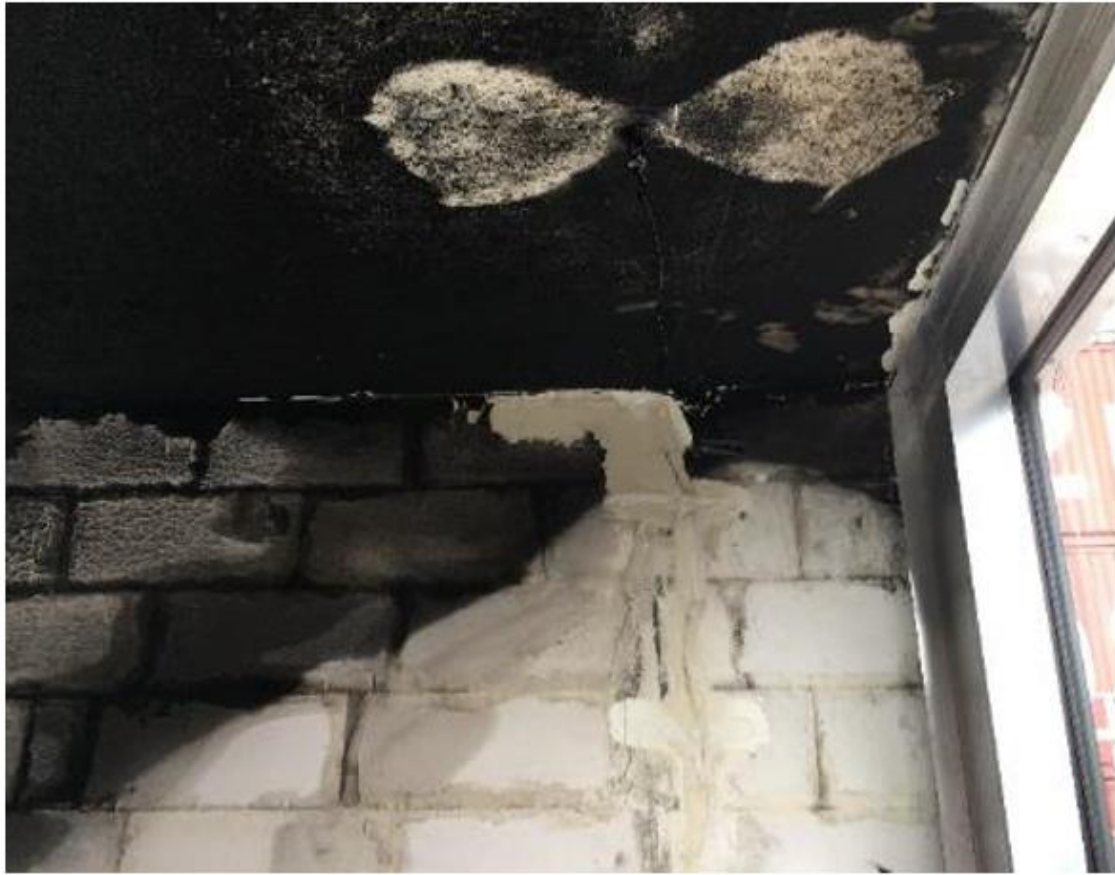
Figure 13. Soot deposition on the walls and the glazing of experiment #4, illustrating the range of water spray coverage in the compartment
