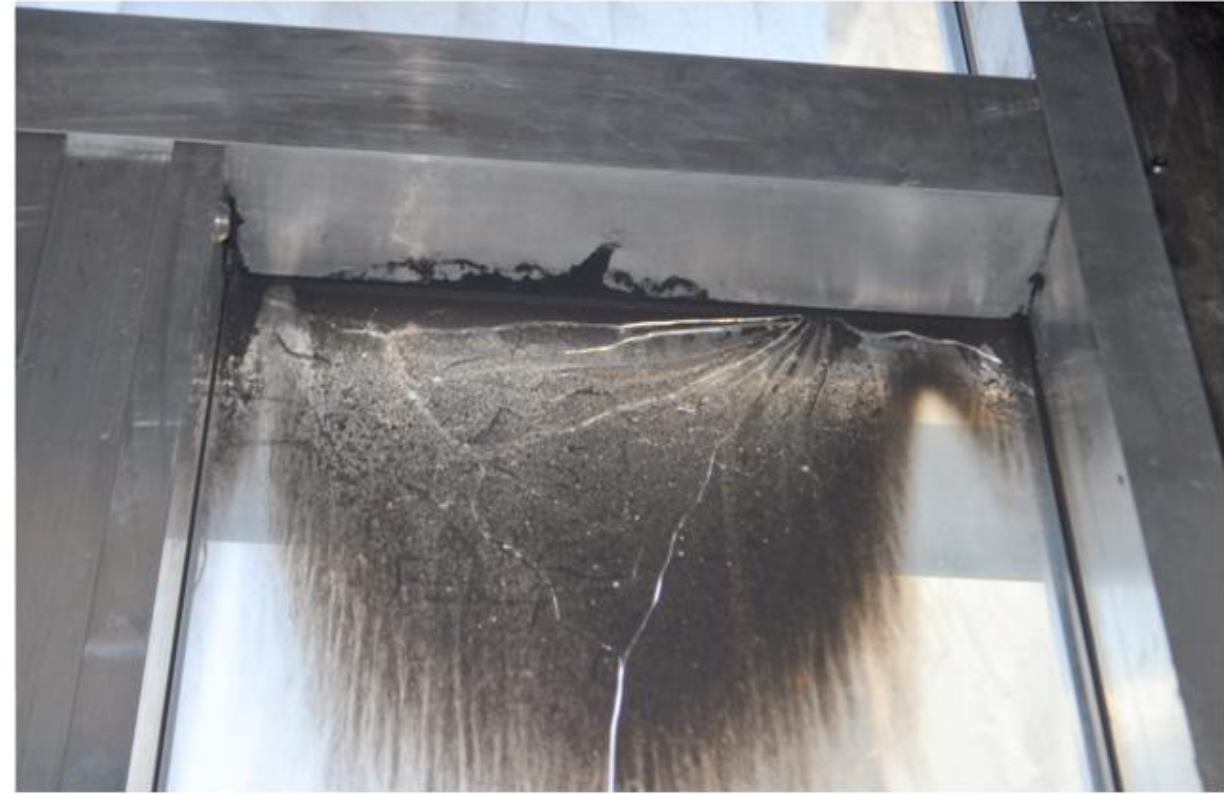
Figure 17. Damage to the test element after experiment #1: cracks are visible in the dry area (covered with soot), while the wet part of the glazing is intact (with the exception of a single vertical crack running through the middle of the element)
