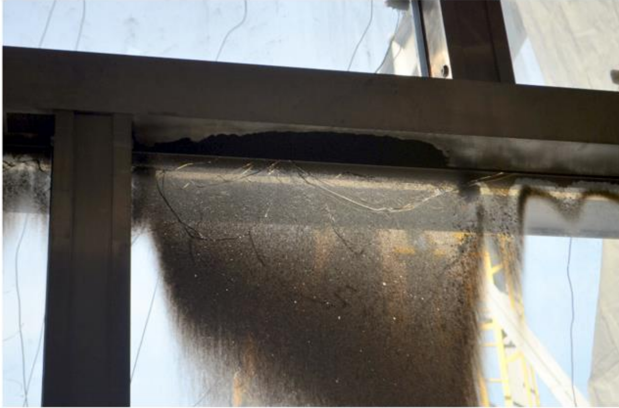
Figure 17. Damage to the test element after experiment #1: cracks are visible in the dry area (covered with soot), while the wet part of the glazing is intact (with the exception of a single vertical crack running through the middle of the element)
