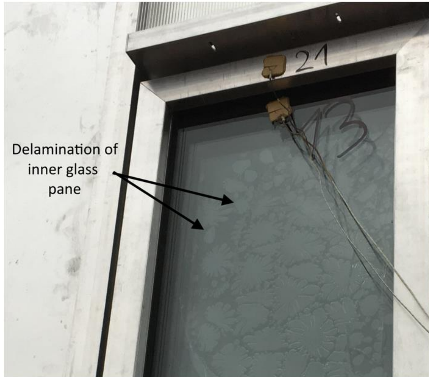
Figure 18. Delamination of the inner glass pane observed after water spray shut-down in experiment #3
