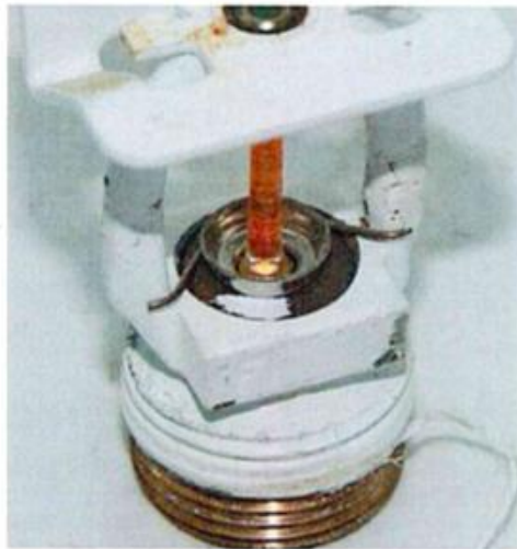
Figure 6 – Specimen 7 Paint daubed on the valve assembly and non-critical areas.
