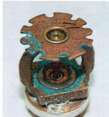
Figure 7 – Specimen 11 Build up of turquoise deposits on The deflector plate, valve assembly and non-critical areas
