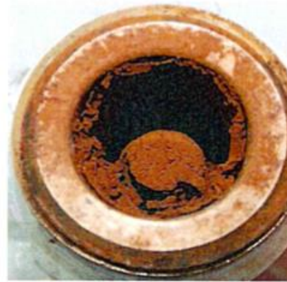
Figure 5 – Specimen 3 Build-up of brown deposits in the waterway
