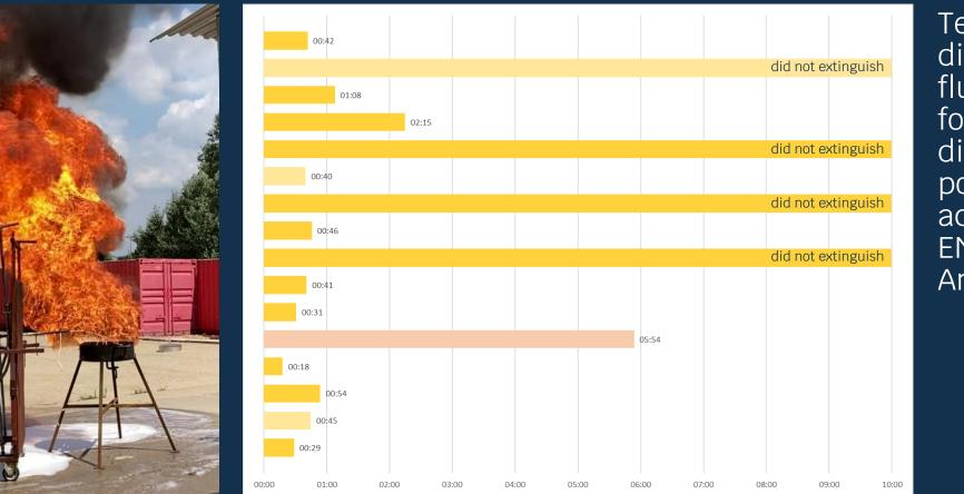
Tests of 3 different fluorine-free foams on 16 different polar fuels according to EN1568-4 Annex I
