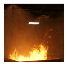
FM5130 non-aspirated sprinkler fire test
