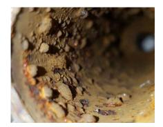
Figure 1: Oxygen corrosion of steel in a closed cooled water system
