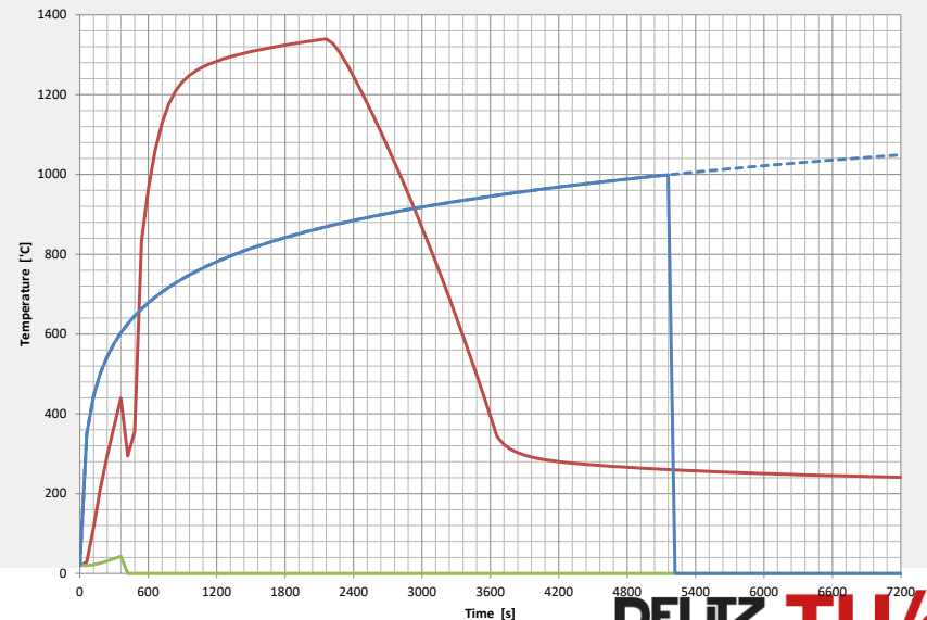
Thermal action by fire (CLT) 86 min SFC
