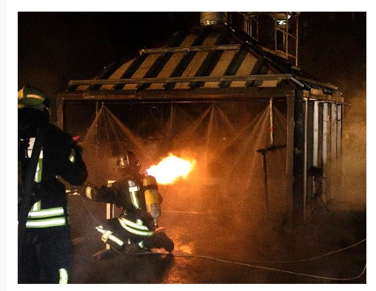
Fire test with lithium-batteries in SUVEREN test chamber
